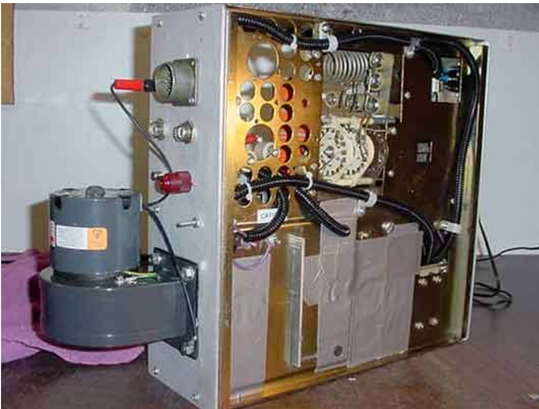
Bottom view, showing blower and holes in former power supply chassis taped over with packing tape to insure all air will pass through the GS-35 cooling radiator.
