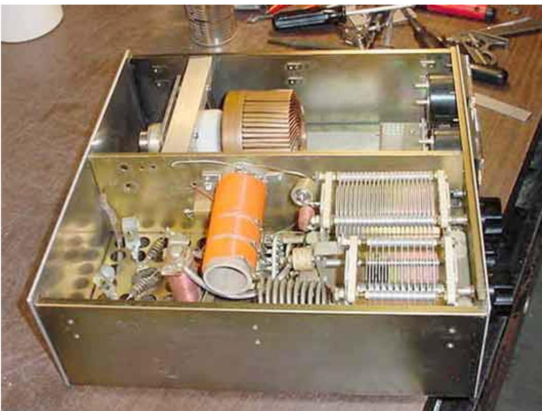
As above, side view, also with additional bracing for GS-35 socket installed.
