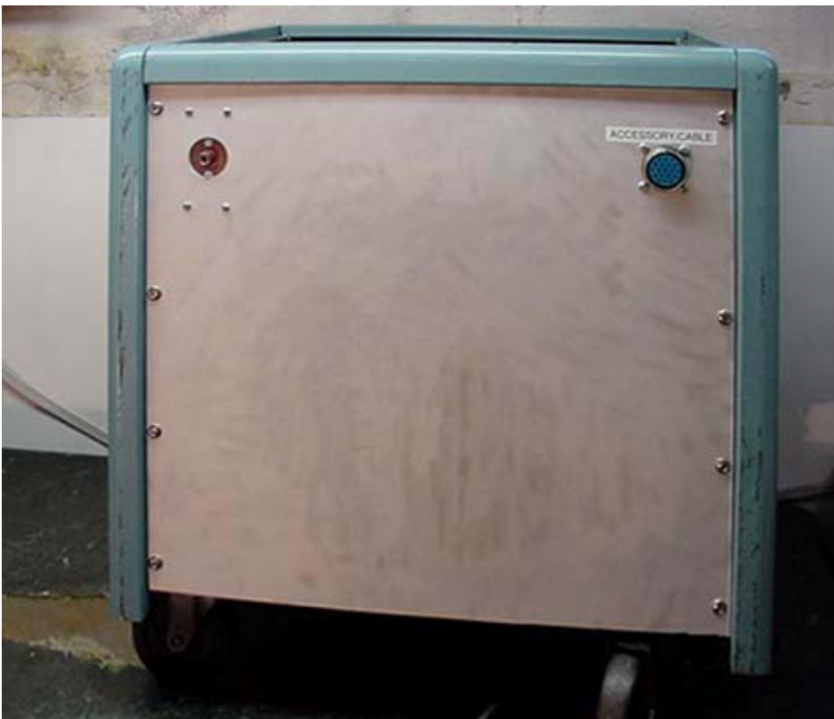
Back view of the cabinet showing the millen HV and control connectors.
