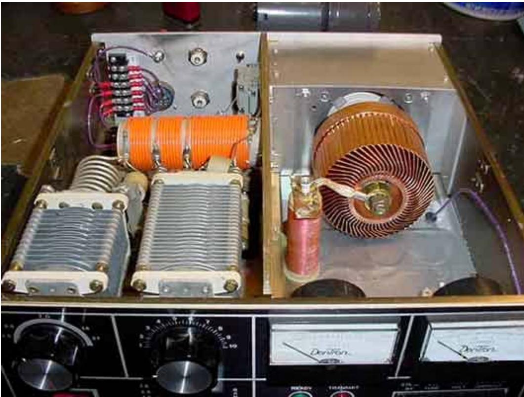
Top view showing tape on TOP of power supply chassis floor as well. The GS-35 socket enclosure has been installed, and wiring of control interface has begun in rear left corner of tank circuit compartment.
