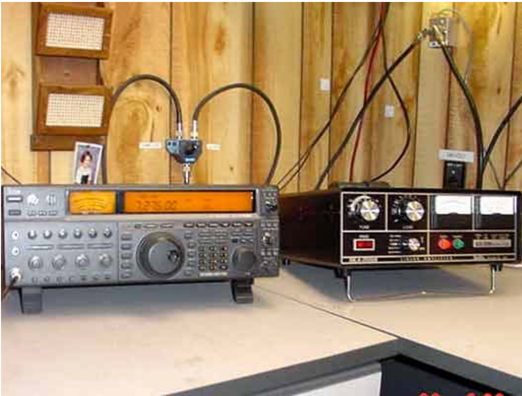
MLA-2500 GS-35B RF deck in-line. The power supply is under the table. Belden 40 KV HV cable and millen HV conectors are used for HV connections.
