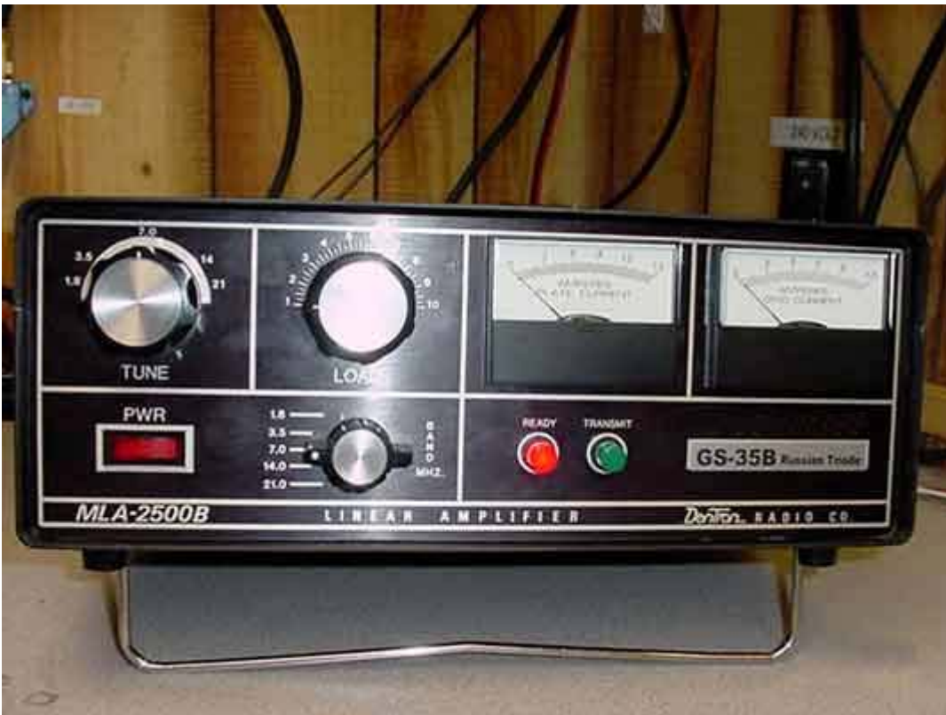
MLA-2500 with meter switches removed and meter swapped out; 1.5A for plate current, 1.0A for grid current - probably could use 0.5A for the grid. Note nifty name plate to cover holes left when switches were removed.
