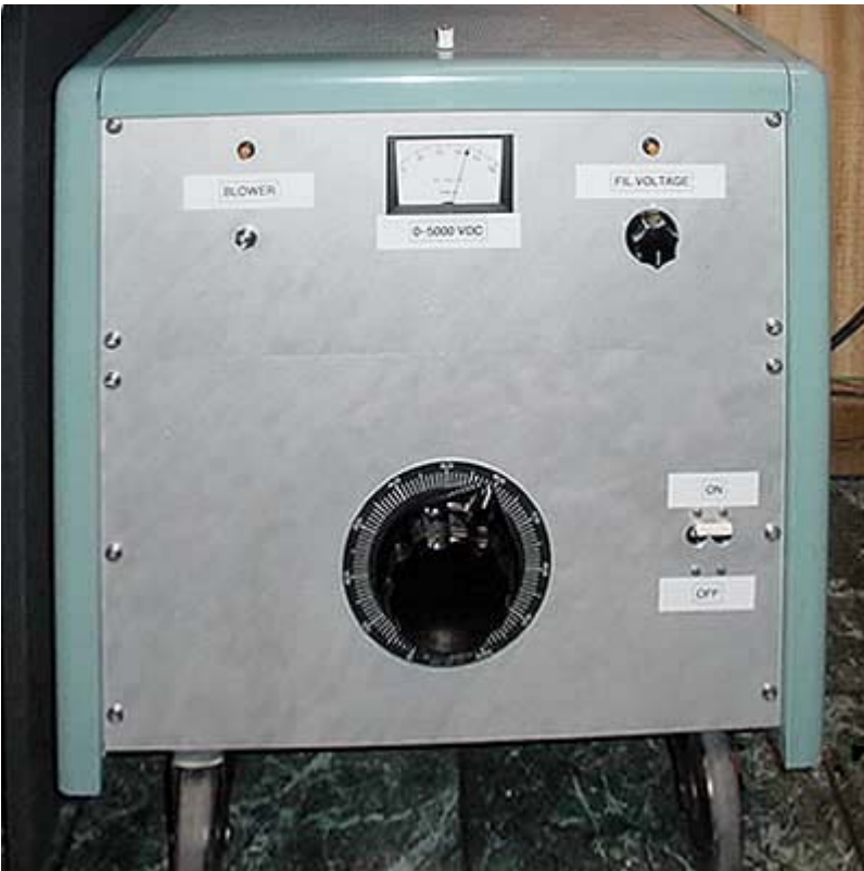
Front view of the remote power supply suitable for GS-35B PAs. The meter is Simpson 0-5000 VDC.
