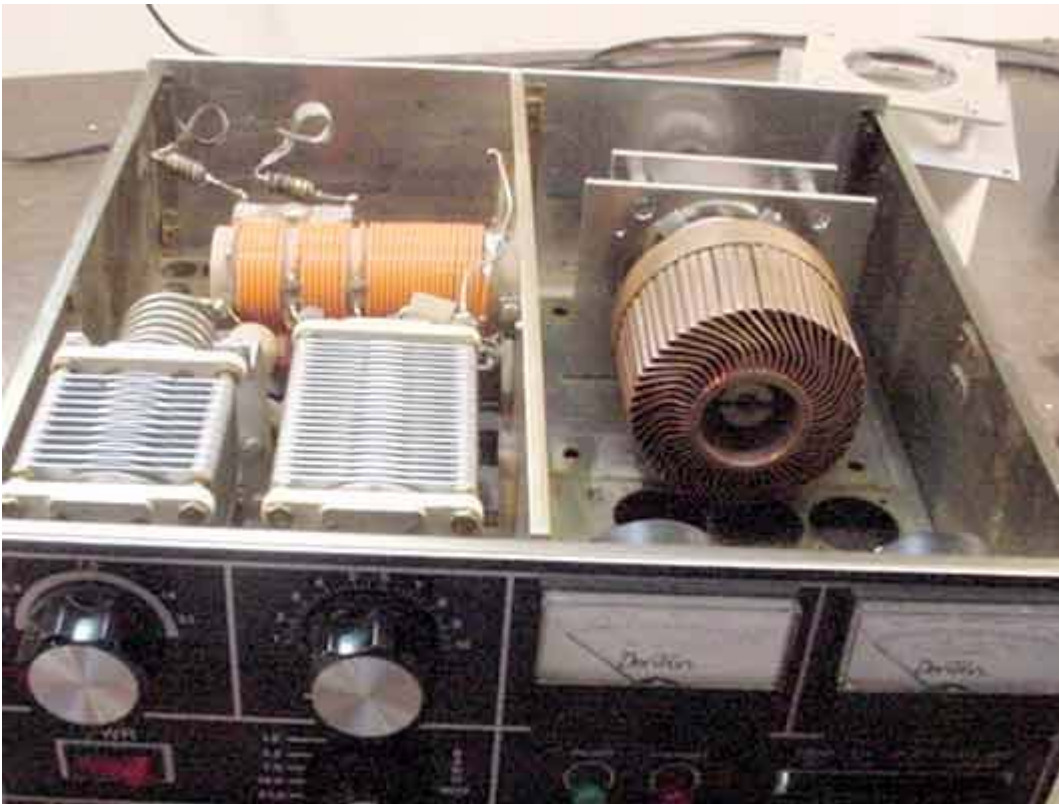
MLA-2500 with original tubes removed, power supply removed, and GS-35 socket installed in former power supply compartment.
