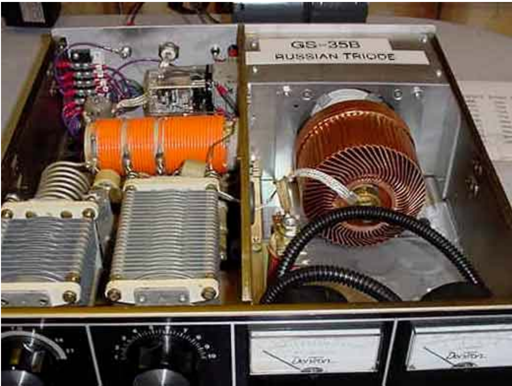
As above, showing more cabling added in tube / metering compartment. The big black cables are actually split flexible cable sheathing.
